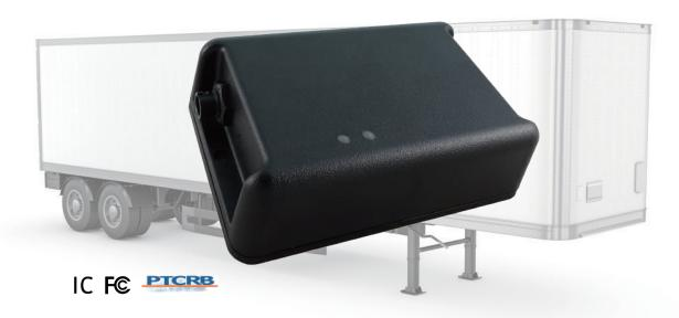
AS11 is equipped with rechargeable battery making it an ideal solution for asset management. With IP68 rated casing, AS11 is designed to operate under extreme environment against water and dust. It is also equipped with GPIOs for varieties of application expandability and flexibility by connecting to a wide range of accessories.
